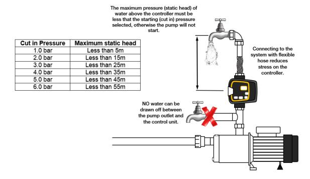
Note: The controller provides dry-run protection in both modes.
